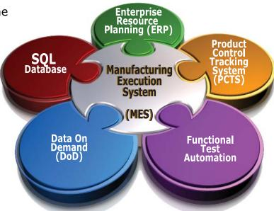
**Data On Demand (DoD)**: DoD is used to communicate and analyze scanned data from the PCTS and Functional Test Automation modules both internally and externally. This information is refreshed every 60 seconds and made available on an interactive company intranet site, as well as on production floor display stations. The collected data maps work-in-progress and completion status for all work orders and reports functional test status and assembly time.
